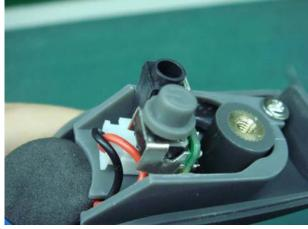
**Step 5.** Install the bottom cover of handheld unit This step is difficult. The hint is to fix one side of the bottom cover firstly, then the other side. However, it needs practice.
