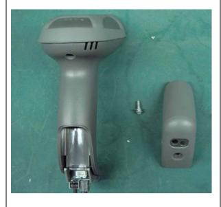
**Step 3.** Insert the battery. Leads the cable going through the groove.
