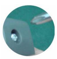
**Step 2.** Remove the bottom cover of the handheld unit.
